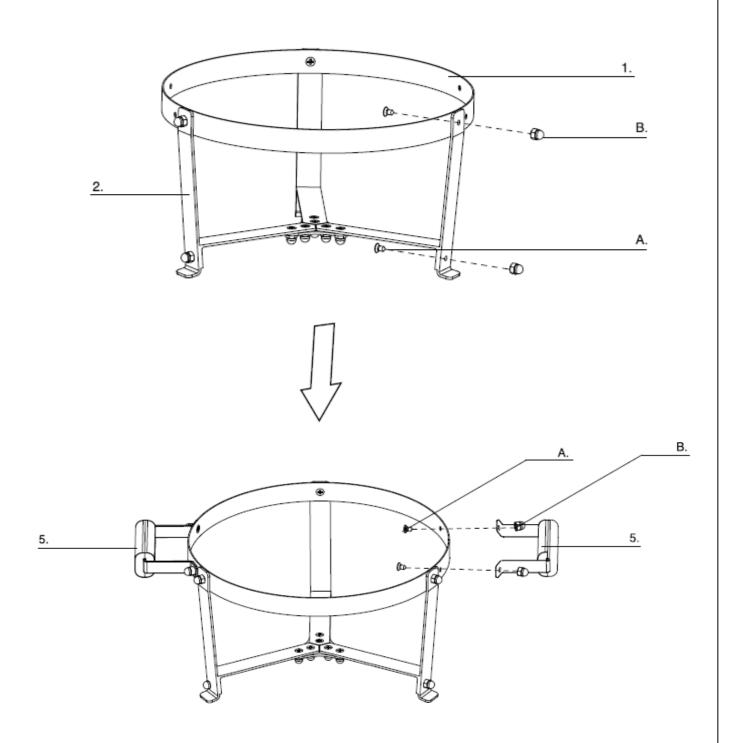
**STEP 3:** To attached the 2x handles(5) to the lid of the brace ring(1), start by aligning the bolts hole of the handles to pre-installed bolts on the lid. Secure the handle(5) with the 2x pre-attached dome headed nuts.
