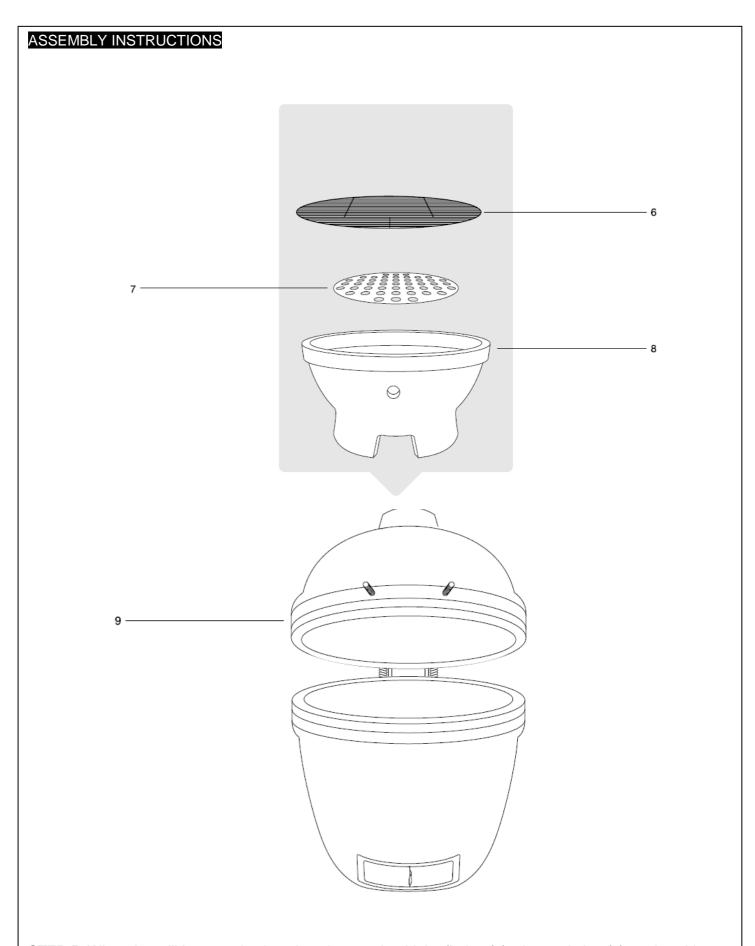
**STEP 5:** When the grill is securely placed on the stand, add the firebox(8), charcoal plate(7), and cooking grill(6) inside the Kamado grill as displayed in the assembly diagram.
