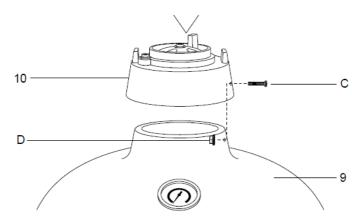
**STEP 7:** To attached the to vent(10) to the Kamado grill(9) place it on top and align both the bolts holes. Secure using 2x bolts(C) and nuts(D). Ensure that the top vent bolt is on the left hand side when assembling it.
