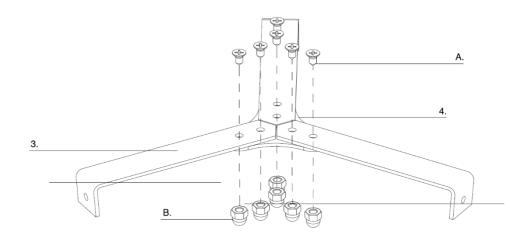
**STEP 1**: Secure the 3x bracket (3) and triangle connection piece(4) by using the 6x screws(A) with the 6x dome headed nuts(B)
