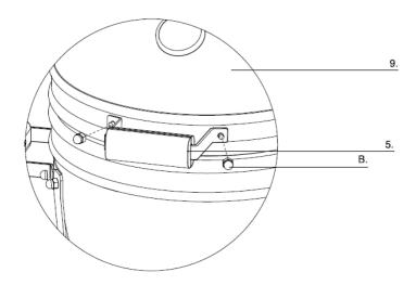
**STEP 6:** To attached the handle(5) to the lid of the Kamado grill(9), start by aligning the bolts hole of the handle to pre-installed bolts on the lid. Secure the handle(5) with the 2x pre-attached dome headed nuts.
